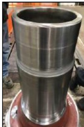
Planetary Gear Shaft wear repair with VRC's high-pressure cold spray system.
