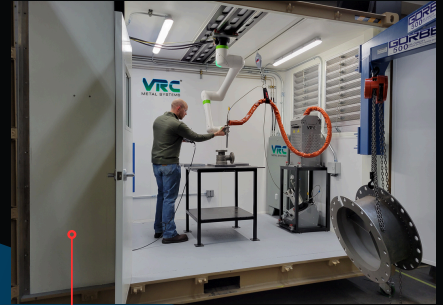
Cold Spray Booth
